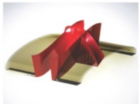
Helicoidal sections through the oblique barrel vault
