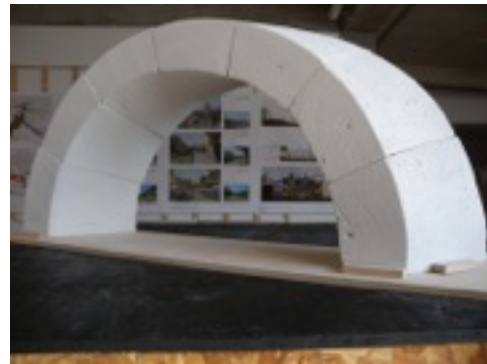
Model of skew arch biais passé made by students at the University of Minnesota
